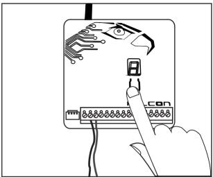
2. Set the serial port format on the Falcon unit to DSC Neo. To do this, remove power from the Falcon, hold down the push-button and re-apply power. Push the button to cycle through the panel serial port format options until you reach the DSC Neo format, indicated by a small letter "d". Release button. The Falcon will remember the new serial port format.
