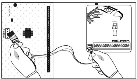
1. Connect the Falcon to the DSC Neo panel through the serial port (PC LINK 2) using the serial cable and adapter marked "DSC Neo" provided. Note that the adapter <u>must</u> be connected to the panel's serial port.
