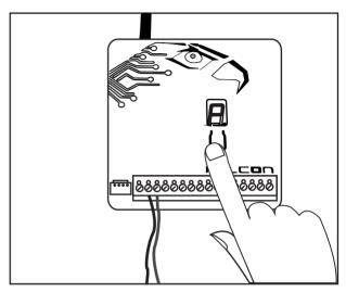
2. Set the serial port format on the Falcon unit to Paradox. To do this, remove power from the Falcon, hold down the push-button and re-apply power. Push the button to cycle through the panel serial port format options until you reach the Paradox format, indicated by a capital letter "P". Release button. The Falcon will remember the new serial port format.
