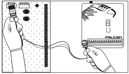
1. Connect the Falcon to the Paradox panel through the serial port using the serial cable and adapter marked "PARADOX" provided. Note that the adapter <u>must</u> be connected to the panel's serial port.
