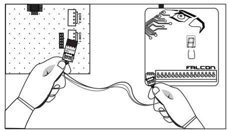
1. Connect the Falcon to the Texecom panel through the serial port (COM 1) using the serial cable and adapter marked "TEXECOM-IDS" provided. Note that the adapter <u>must</u> be connected to the panel's serial port.
