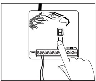
2. Set the serial port format on the Falcon unit to Texecom. To do this, remove power from the Falcon, hold down the push-button and re-apply power. Push the button to cycle through the panel serial port format options until you reach the Texecom format, indicated by a small letter "t". Release button. The Falcon will remember the new serial port format.
